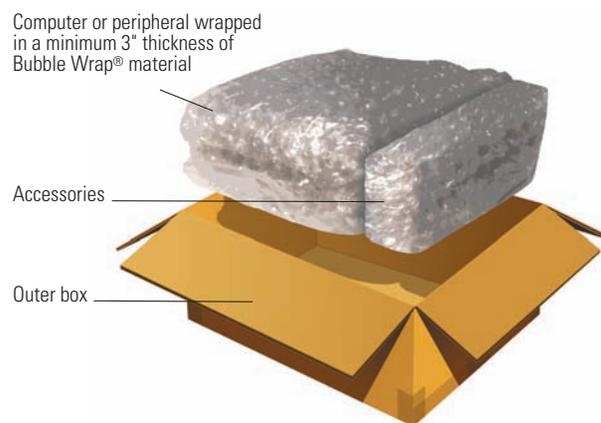
Wrap the computer or peripheral on all sides with at least 3" to 4" of air-cellular cushioning material such as Bubble Wrap®. Place the wrapped item inside a sturdy outer box. Accessories that are wrapped in appropriate amounts of cushioning can also be placed in any open spaces of the box. Fill all spaces with additional cushioning so that the wrapped item fits tightly inside the box. If no open spaces exist, pack accessories in an additional box.
