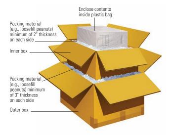
Since this type of packing material allows the packaged item to settle to the bottom of the box, it is important to use the overbox method of packaging. The inner box should be at least 4" greater in length, width and height than the item you are shipping. This will allow for 2" of space for all six sides. The outer box should be at least 6" greater in length, width and height than the inner box. This will allow 3" of space between the inner box and the outer box.
