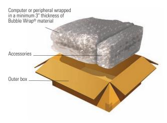
Wrap the computer or peripheral on all sides with at least 3" to 4" of air-cellular cushioning material such as Bubble Wrap<sup>®</sup>. Place the wrapped item inside a sturdy outer box. Accessories that are wrapped in appropriate amounts of cushioning can also be placed in any open spaces of the box. Fill all spaces with additional cushioning so that the wrapped item fits tightly inside the box. If no open spaces exist, pack accessories in an additional box.
