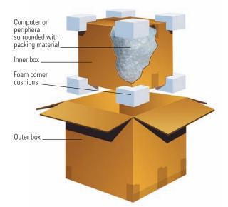
You may choose to use foam corner cushioning specifically designed to properly cushion your product during shipping. This packing method allows you to use one size of inner box, one size of outer box, and one type of foam corner cushioning to ship items of various sizes and weights.
