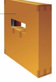
This design combines the use of a scored pad, a die-cut corrugated insert and a molded insert to help provide cushioning and bracing of the door inside the outer shipping container.
