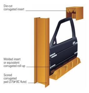
Die-cut full-overlap top-load corrugated outer container (275# BC flute) \_\_\_\_\_
