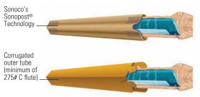
This rigid outer package design protects the pre-paint trim or moldings from scratches and bending.
